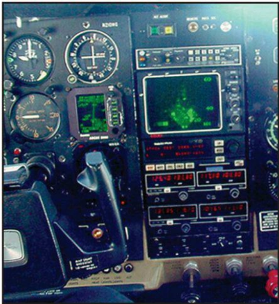
The radar screen can be seen in this in-flight picture. It is picking up some rain which is visible in the lower
