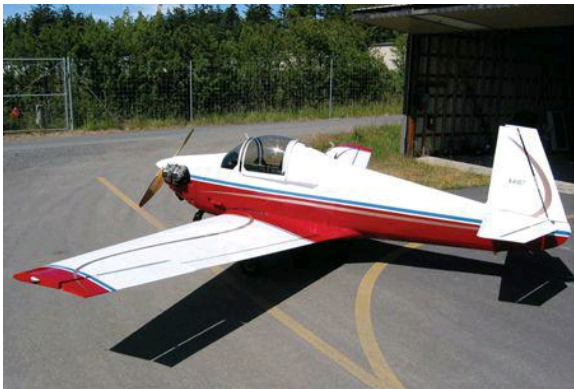
Airplane #8: 1955 Mooney M-18C-55, Continental 65-horsepower, retractable landing gear, 120 mph, one-seat, purchased December, 1995, sold June, 2006. Flown 530 hours. Restored, 2003. “Best of Class, less than 80 hp” AirVenture, 2003.
